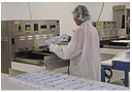
Tray sealing at Life Science Outsourcing, Medical Package Testing Div. is followed by in-line leak testing in the facility's cleanroom.
